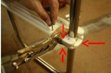
6. Clamp the fork in place, making sure that one set of front and back bolt holes is visible and accessible. Push the drill bit or a nail through the bolt holes to mark the locking fork.
