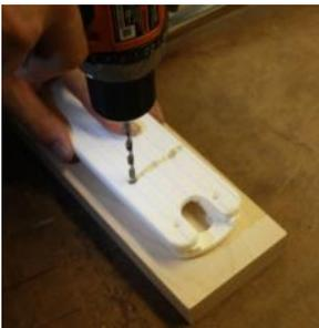
9. Place a bolt through one of the drilled holes to lock the fork and drill all four holes for the fork.
