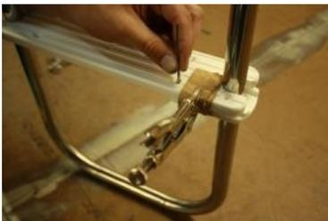
7. Remove the fork and tread from the rung. Reassemble the rung and fork for drilling, making sure that the holes in the tread line up with the drill-bit marks on the forks.
