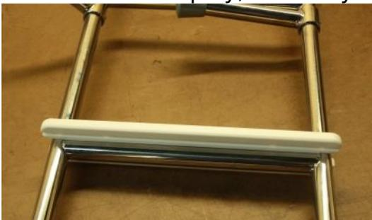
3. Slide one of the locking forks around the vertical rails below the rung with the tread.
